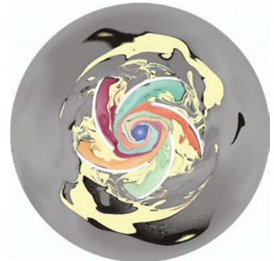
Figure 9: Advecting structured patterns reveals additional transport information about the flow. We applied an forward advection of a 2D texture projected into the flow volume. In the resulting image we can see in which section one point in the texture would end up after a variable integration time in one slice at z = 0.02 . The first image shows the original pattern. In rows 2 to 4 this texture is advected to the time steps 26, 52 and 80 for each simulation model. We see the impact of the turbulence and evolving vortical patterns at the section boundaries. These images show clearly the differences between the simulation models. At time step 26 we see evolving the first vortical structures and also the beginning of the distribution of the inflow of the channels. At time step 52 it becomes visible that in the SAS the inflow of channels 1 and 4 block the inflow of the other channels, which is not the case using DES an SST. In all three models we can also see that some areas of the outer region move back into the transport area and even into the channels. At time step 80 the fully evolved transport pattern is shown. The images reveal large recirculation structures behind the rotor blades, especially in channel 3 and 5 of the SAS model.
